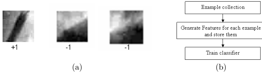
Figure 2. Examples of positive and negative examples used for training (a). Steps used in training for classifier (b)
