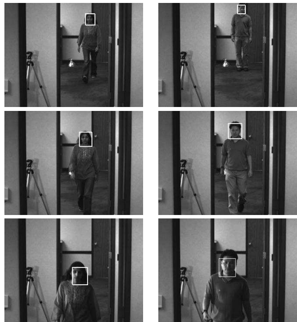
Fig. 2. Face tracking using PF-MT as the individuals walk through different lighting conditions. The white box shows the image region corresponding to MMSE estimate of the “shape vector”.
