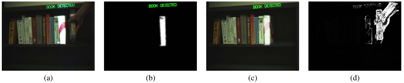
Figure 3: Foreground segmentation in the presence of augmented imagery. (a) Scene containing overlaid projected information as well as “real” change. (b) Framebuffer contents of the projector after they have been warped and color corrected for the left camera. (c) Synthetic expected image constructed after combining warped and corrected framebuffer contents with background model. (d) Detected differences.
