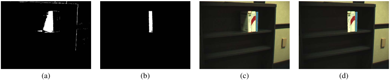
Figure 4: Images of a bookshelf taken when a book is added. (a) Foreground image detected using the previous state of the bookshelf. (b) Foreground image after eliminating non-spine pixels using (3) (c) Bounding box BL_j computed from (c) superimposed on the foreground image for computation of the histogram HL_j for the book j . (d) Updated state of the bookshelf as described by (5).
