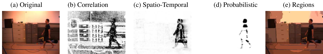
Figure 1: From left to right: Image 120 of MIT Indoor sequence; Output of a correlation filter (Sec. 2.2.1); of a spatio-temporal filter (Sec. 2.2.2)(negated to be more visible); of a probabilistic filter (Sec. 2.2.3)(negated to be more visible); region segmentation (Sec. 2.2.5).
